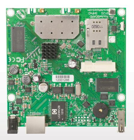
The RB912 is a small wireless router with an integrated high power wireless card and an additional miniPCle slot for 802.11 wireless, or 3G card. The Gigabit port helps to utilize the full potential of 802.11n wireless speeds.
